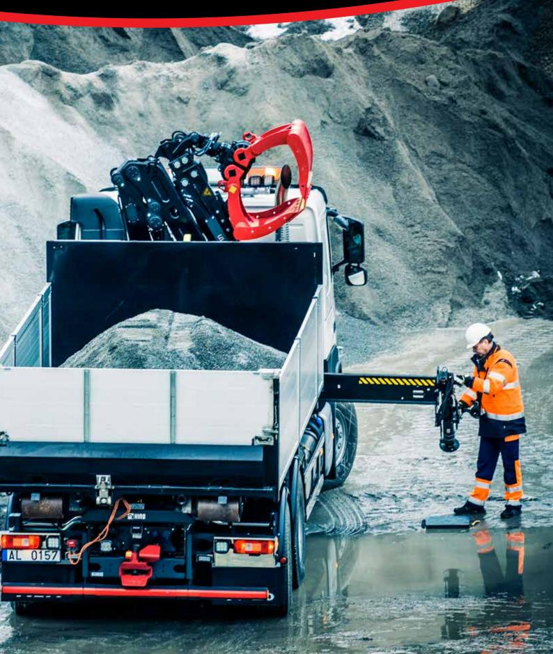
When you finish a job, you want to move straight on to the next. This is why cranes in the new HIAB Z-series fold neatly behind the cabin – with the bucket still attached.
