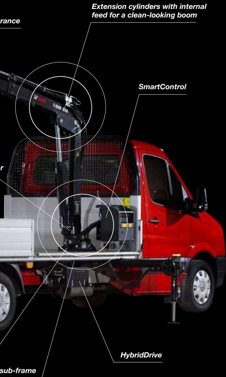
Extension cylinders with internal feed for a clean-looking boom
