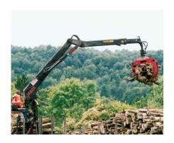
The **J1620Z** is a crane proven in the field in rugged use, enduring continuous, hard work. Designed mainly for loading cutto-length timber, the J1620Zpossesses enough lifting capacity to handle full-length stems. Its narrow boom assembly enables an unrestricted view from its ergonomic control position over the entire work area.
