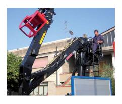
The **J1440Z**, folding into a compact space, is a crane more powerful than its size class, effortlessly loading even the heaviest timber. Its advanced Z design features high performance, guaranteed by its powerful double-slewing system and the Power Link, which improves close-range lifting capacity.
