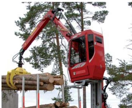
The efficient **J1080S** equipped with a powerful double slewing system has been designed for those who do abundant loading of timber. In the crane construction, easiness of maintenance has been paid great attention to, and the new ergonomic control position makes the loading work more comfortable than ever. The crane can be equipped with manual control or digital electric control system.
