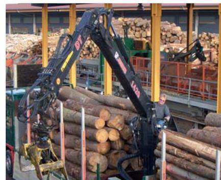
The **J1420S** is the heavyweight of cut-to-length timber cranes, loading timber reliably, efficiently and effortlessly. J1420S is equipped with a separate stabiliser leg framework, increasing installation options and enabling the use of wider stabiliser legs when necessary.
