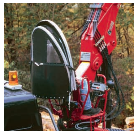
The high seat hood is fastened to the seat at four points.
