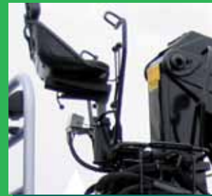
The control valve is located in a sheltered place
